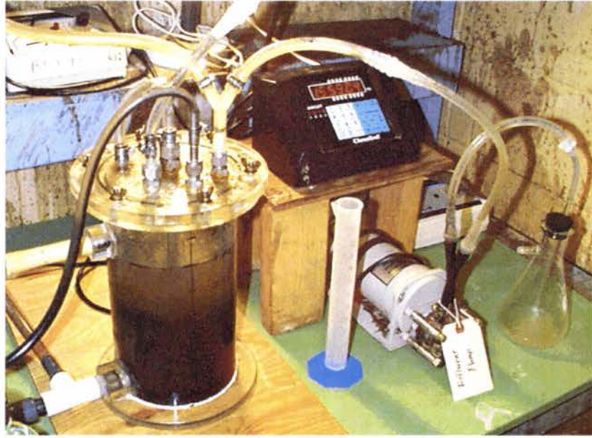
Figure 3. Photo of the Master Culture Reactor (MCR)
